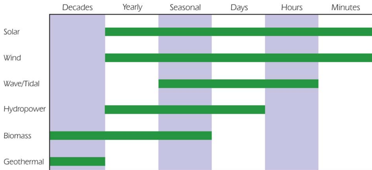
Figure 2: Timescales of natural cycles of renewable energies
